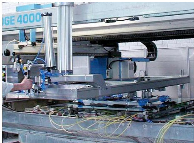
Moving into the inside of the machine, subsequently travelling of the suction frame and positioning of the glass pane in the machine
