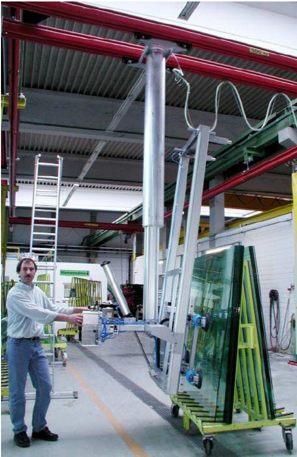
Unloading from glass rack (version: long slide rail)
