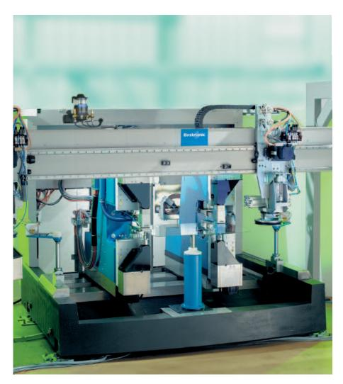
champ'drill is a fully automatic and flexible drilling machine for the processing of automotive glass. The trendsetting technology ensures maximum productivity and a very high level of user friendliness in proven Bystronic glass quality for the user.
