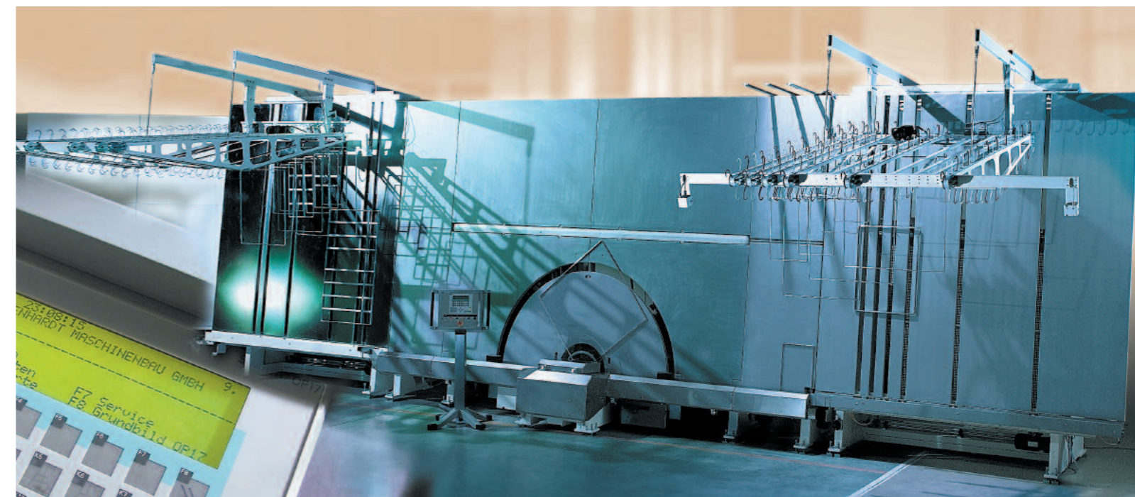
Safe and fast turning of spacer frames, also for spacers with muntin bars (option)
